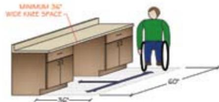
*\*Toe clearance space under a cabinet or appliance is between the floor and 9" above the floor. Where toe clearance is required as part of a clear floor space, the toe clearance should extend 17" minimum beneath the element. (ANSI A117.1 306.2)*
